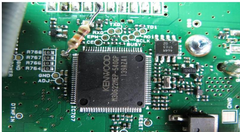
Now take your NPN transistor, bend the leads as shown, lay over IC715 (the AF Amplifier IC) and solder the emitter lead to pin 9. Solder the other end of the 10K resistor you used in the previous step to the base of the NPN transistor.
