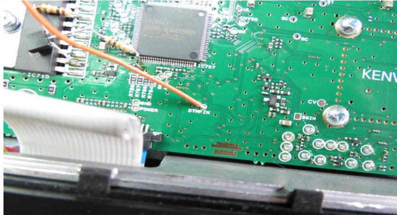
Connect the two wires you soldered to the mic connector on the front panel, to your 4 conductor cable. In our case, PTT (red) goes to red on our cable while TX Audio (yellow) goes to black.
