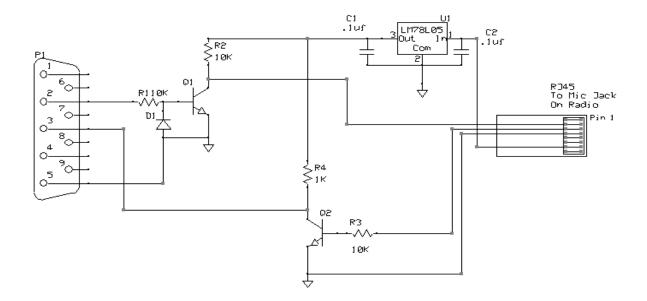
Unfortunately, the A suffix models (the ones sold in the USA) do not have a packet jack already installed and necessary signals, such as PTT, COS and audio, is not readily available from the mic jack. Fortunately however, Kenwood made these signals very easily accessible but it does require you open the radio in order to connect to them.
