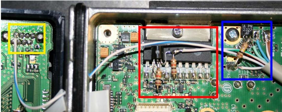
It is not necessary to do both the PL and the COR mods, however I did both so I could have a COR and a PL line to the controller. The audio from the PR9 pad is un muted so you will have COR and receive audio whether you receive correct PL or not. This allows me to disable the PL with a macro by changing the port to Carrier or CTCSS access instead of using the A72 command.
