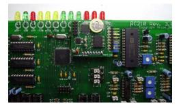
If you have the optional AP1 Intelligent Autopatch, plug its 8 pin connector into the RTC's JP2 connector, taking care to line up pin 1. That's it! Now power up your RC210 and set the clock and calendar (which should be the last time you ever have to do that!)
