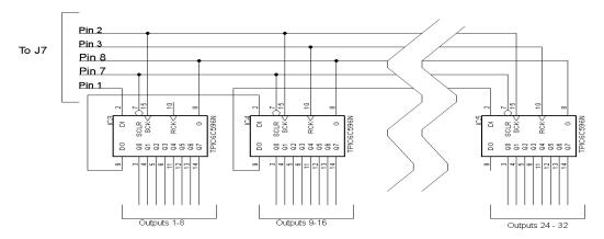
Only some of the stages needed to recover those functions have to be used. Each shift register used adds 8 outputs. So if you only need an additional 32 outputs (above and beyond the 7 "on-board" outputs), you only need add 4 stages. The outputs of the above ICs are open drain JFETS and can directly sink up to 30 volts @ 100 ma.
