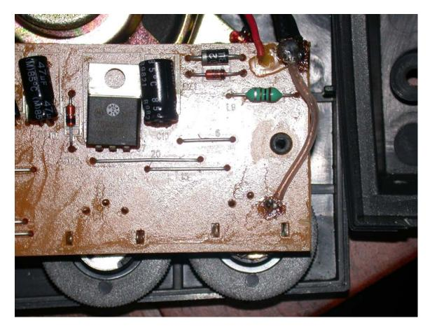
This is a close up of where I connected to the audio. I used shielded line. The center conductor hooks to the vol. pot as shown, and the shield is connected at the point where the negative side of the back up battery connection. I wouldn't worry too much about conditioning the audio, NOAA audio sounds like crap no matter what type radio you listen to it with.
