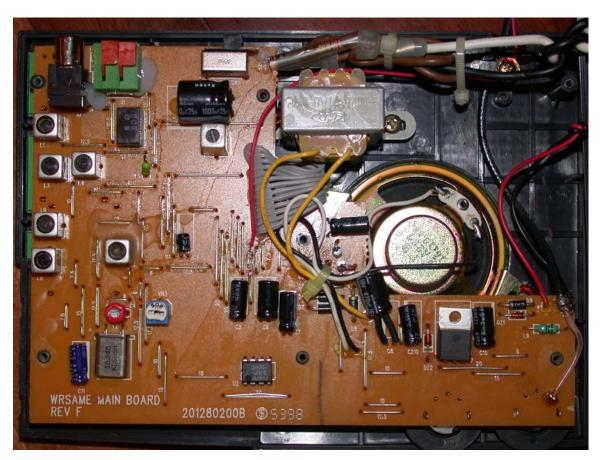
It took the built in antenna off and that is where my wires come out. I use an outside antenna. You may want to use the built in antenna, if so you'll need to drill a hole in the case.
