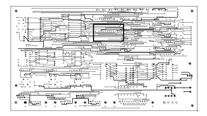
Solder the 22K resistor from Pin 8 to Pin 5 of J5 (version 3.0 board) or J7 (version 2.8) as shown.
