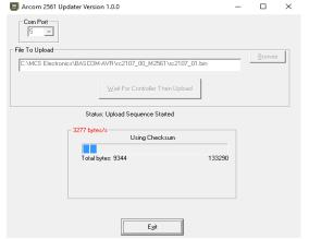
Updater will now automatically start the upload. Notice the Status Line changes to Upload Sequence started and you can watch the progress of the upload in the box below
