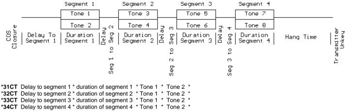
CT refers to the courtesy tone set you wish to program and is entered as 01, 02, 03 and so on, up to 10. The delay and duration parameters are in milliseconds (ms) and the tone parameters are in hertz (hz). The \* separators must be used.
