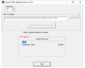
Updater will now automatically start the upload. Notice the Status Line changes to Upload Sequence started and you can watch the progress of the upload in the box below
