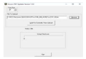
You are now ready to actually upload the update into your RC210. Make sure one end of your serial cable is plugged into the correct com port on your computer and the other end is plugged into the RC210's serial connect (via the adapter cable). Click the Wait for Controller Then Upload button
