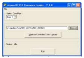
You are now ready to actually upload the update into your RC210. Make sure one end of your serial cable is plugged into the correct comport on your computer and the other end is plugged into the RC210's serial connect (via the adapter cable). Click the Wait for Controller Then Upload button
