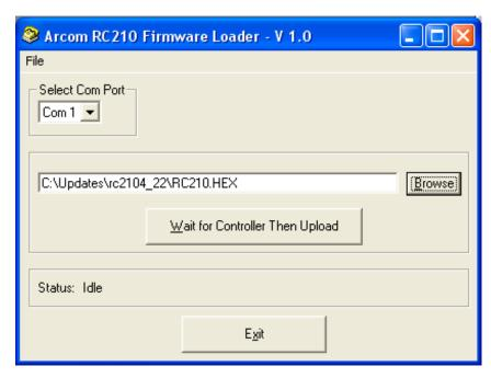
You are now ready to actually upload the update into your RC210. Make sure one end of your serial cable is plugged into the correct com port on your computer and the other end is plugged into the RC210's serial connect (via the adapter cable). Click the Wait for Controller Then Upload button
