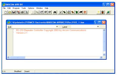
You will see a new window with the version number of the firmware. You are now ready to actually program your RC-210. Make sure the programming cable is plugged into your computer's printer port (the one you selected earlier) and your RC-210. The RC-210 may be left powered up while connecting the cable. Temporarily remove jumpers JP15 and JP16 (this removes the serial driver from the circuit to avoid interference issues)
