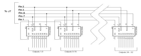
Only some of the stages needed to recover those functions have to be used. Each shift register used adds 8 outputs. So if you only need an additional 32 outputs (above and beyond the 7 "on-board" outputs), you only need add 4 stages. The outputs of the above ICs are open drain JFETS and can directly sink up to 30 volts @ 100 ma.
