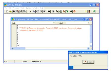
When the write cycle is over, you'll see a new window pop up. This indicates the program write is being verified as ok. Once this is done, the window should close. If you have no errors, your RC-210 should automatically reset and announce its signon message. You are now ready to go with the updated firmware!
